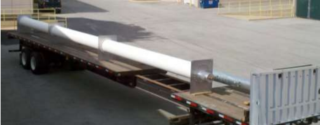
Elliptically Polarized Direction Side Mount Antenna –VHF with Support Mast Elliptically Polarized Skull Pattern with 35% V-POL. Installed 8/10/12
